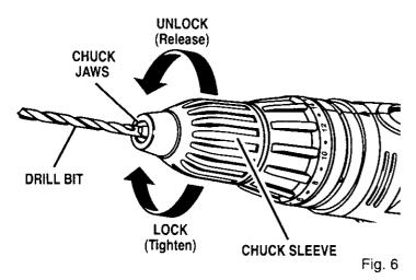
**WARNING:** Do not hold chuck sleeve with one hand and use power of the drill to tighten chuck jaws on drill bit. Chuck sleeve could slip in your hand or your hand could slip and come in contact with rotating drill bit. This could cause an accident resulting in serious personal injury.
